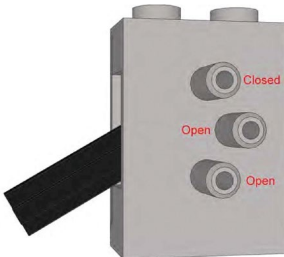
Figure 10-5. This LEGO air switch in the down position opens the middle and lower ports
