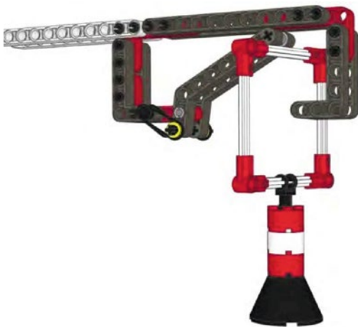
Figure 8-8. When the carabiner makes contact with the loop, the latch opens
