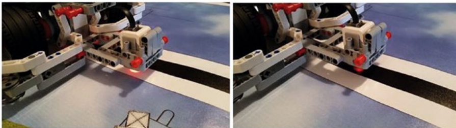
Figure 5-4. Calibrating the DemoBot Color Sensor over a light area (left) then over a black line (right)
