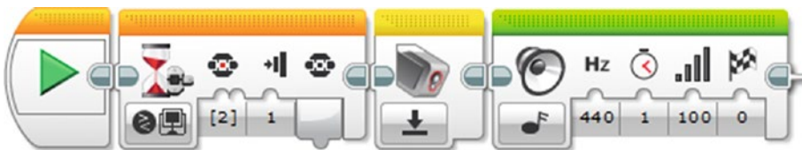
Figure 5-8. A program to delete the current Color Sensor calibration
