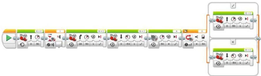
Figure 13-2. With uncommented EV3 code, the flow is hard to understand
