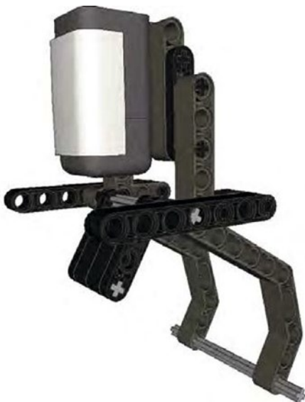
Figure 7-12. With the bumper pushed the black beams are removed from the view of the Color Sensor
