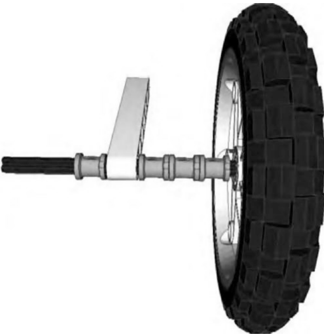
Figure 2-18. Multiple bushing spacing on a wheel axle, moving the wheel farther from the chassis and causing more friction
