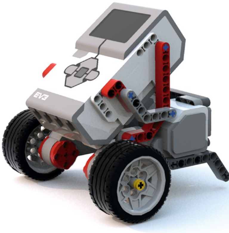
Figure 2-20. A two-wheeled robot with skids in the rear for balance
